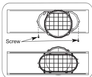
Insert the screw in the hole in the window exhaust adapter to prevent the window exhaust adapter from sliding out of the vent opening.
