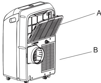
A.Evaporator air intake filter panel door
