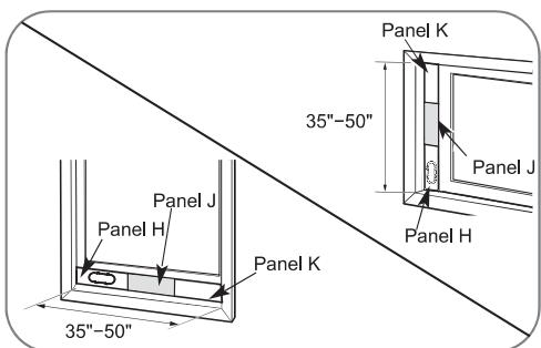
For window openings from 35" to 50", use the window vent panel and two extension panels (Panel K and Panel J).
