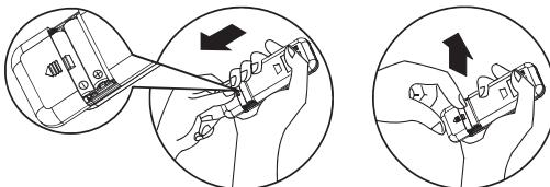
2. Insert new batteries making sure that the (+) and (-) of battery are matched correctly.
