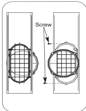
Insert the screw in the hole in the window exhaust adapter to prevent the window exhaust adapter from sliding out of the vent opening.
