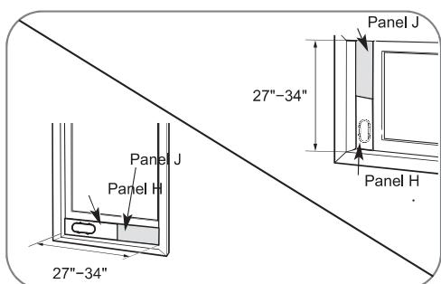
For window openings from 27" to 34", use the window vent panel(Panel H) and a extension panel (Panel J).
