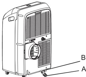
A.Primary drain cover B.Primary drain plug
