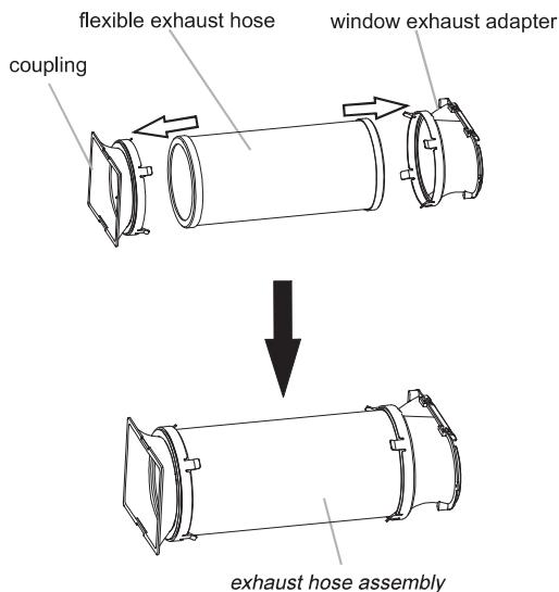
3. Insert the coupling into the slot on the back of the air conditioner.
