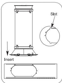
Align the tabs on the window exhaust adapter with the slots in the vent panel.
