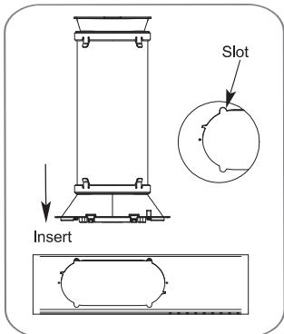
Align the tabs on the window exhaust adapter with the slots in the vent panel. Insert the window exhaust adapter into the opening in the vent panel.
