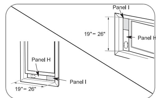
For window openings from 19" to 26", use the window vent panel(Panel H) and a extension panel (Panel I).
